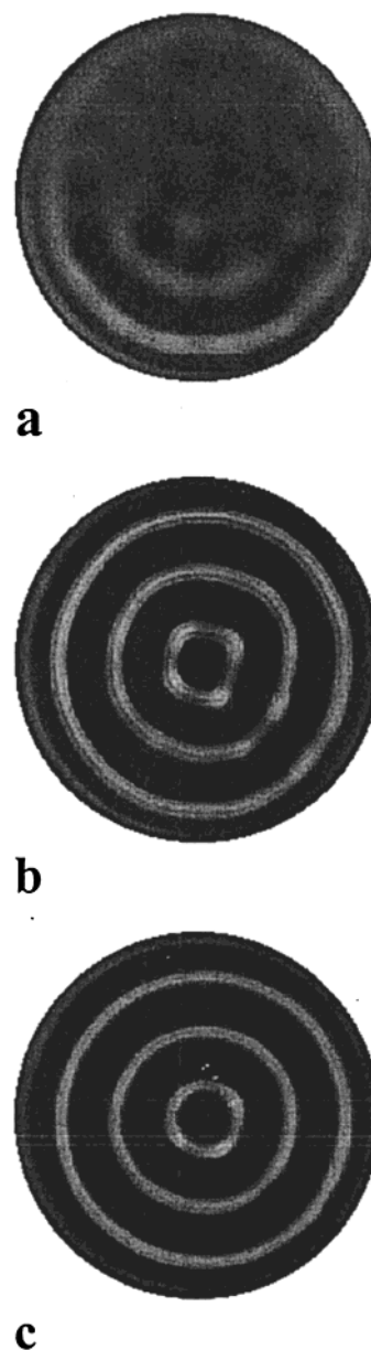
Figure 4. Evolution of convection patterns generated in MAOP-PDMS layers: (a) \Delta T = 3.89 °C, (b) \Delta T = 5.03 °C, and (c) \Delta T = 6.81 °C. d = 0.3096 mm.
